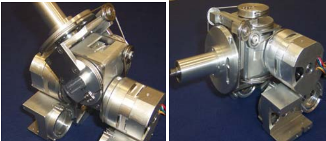
Fig. 5 The compact mechanical design of the differential 3DOF iCub waist.
